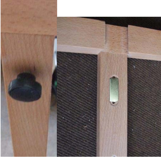
2. Black knob and backing plate placed behind mast to minimise movement. The plate is the same as used on canvas support. The black knob has a longer bolt. (5.2cm incl knob)
